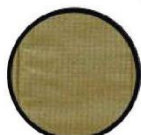
CAPA EXTERIOR Outer Shell PBI GEMINI XTL (40% PBI®/ 60% Kevlar®)
